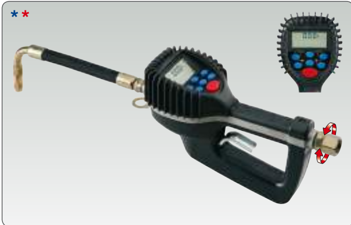
Art. 37704 Digital dispensing oil gun with preselection, equipped with: - inlet swivel joint F 1/2" - adjustable rigid terminal - automatic closing nozzle \varnothing 16 mm
